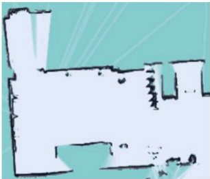
The map scanned by the robot's laser
