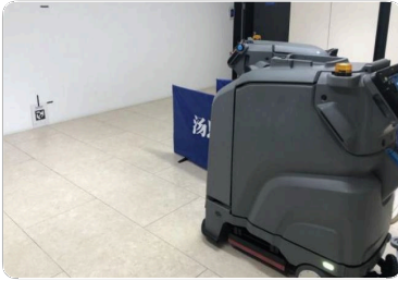
Front monocular scanning (Robot needs to be facing the QR code)
